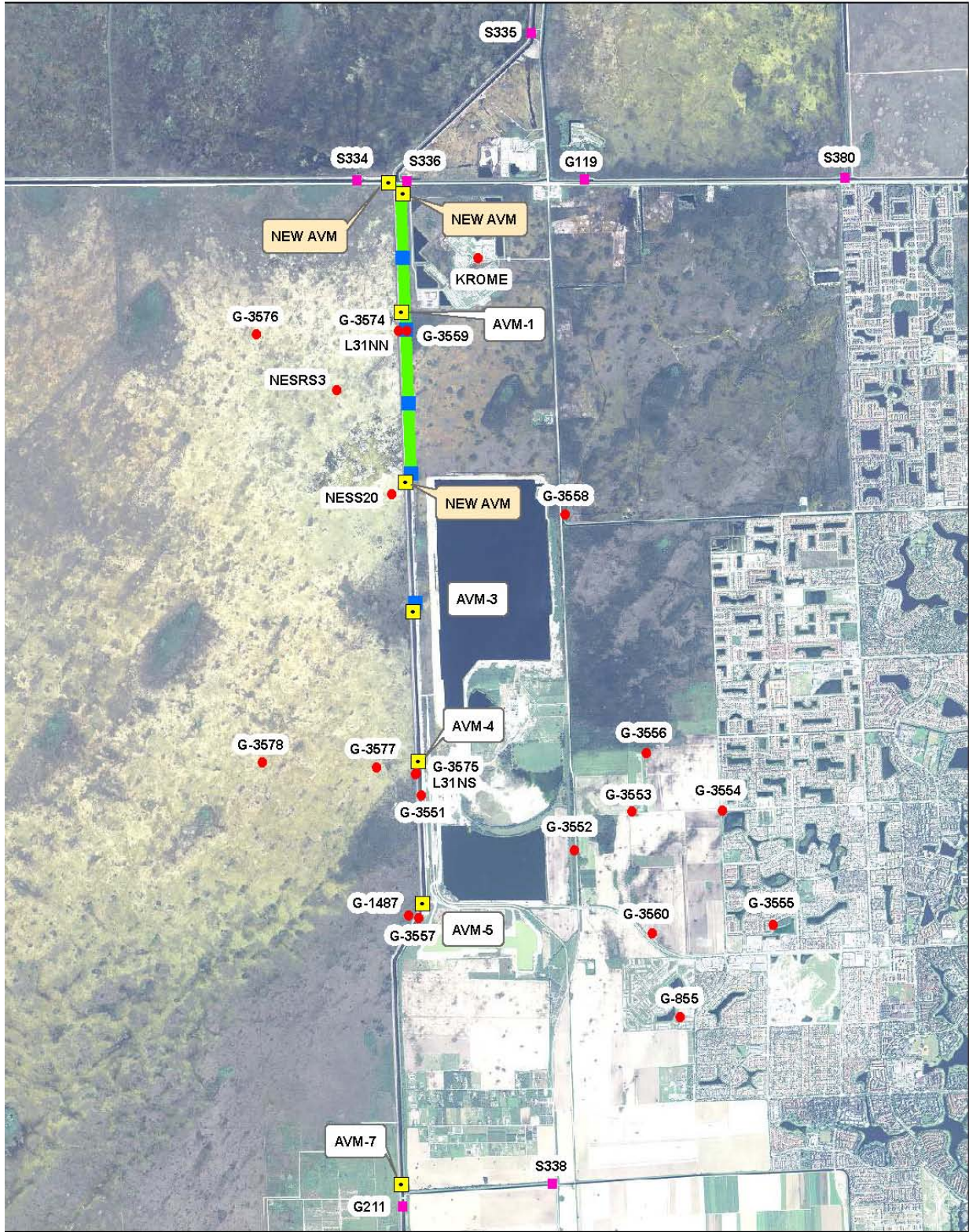
Figure 1. Monitoring Plan location map. The green line represents the 2-mile seepage barrier and the blue squares represent the proposed shallow upgradient and downgradient monitoring wells.
