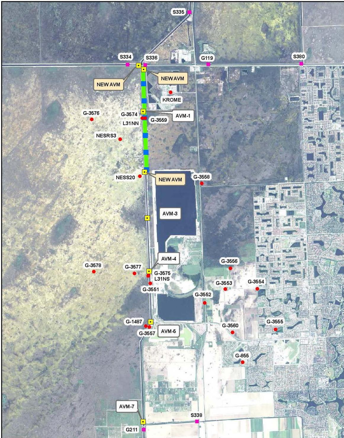
**Figure 4.** Monitoring Plan location map. The green line represents the 2-mile seepage barrier and the blue squares represent the proposed shallow upgradient and downgradient monitoring wells.
